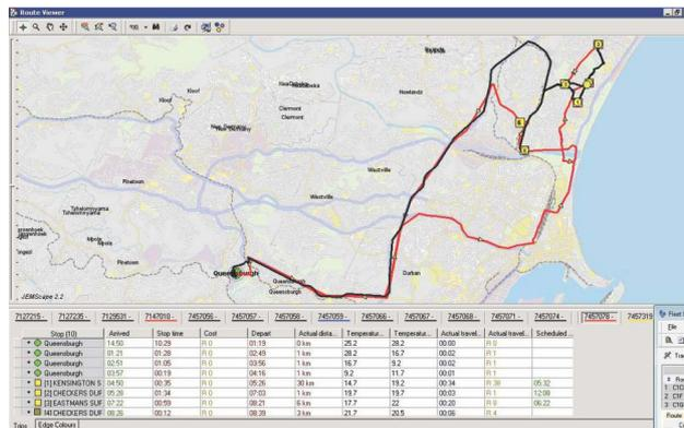
FLO lets the controller overlay the scheduled route with actual tracking data generated from the GPS system, flagging unauthorised stops and extreme route deviations.
